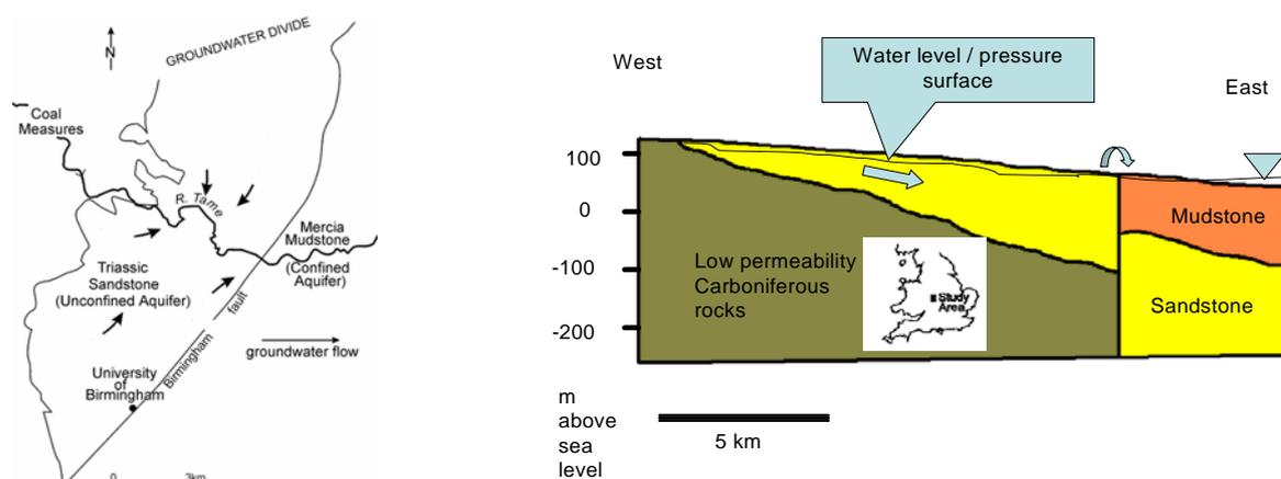
**Fig. 1:** Outline geological map (with generalized groundwater flow directions) (left) and section (right) of Birmingham. City covers entire area shown on map. From Tellam (In Press).
