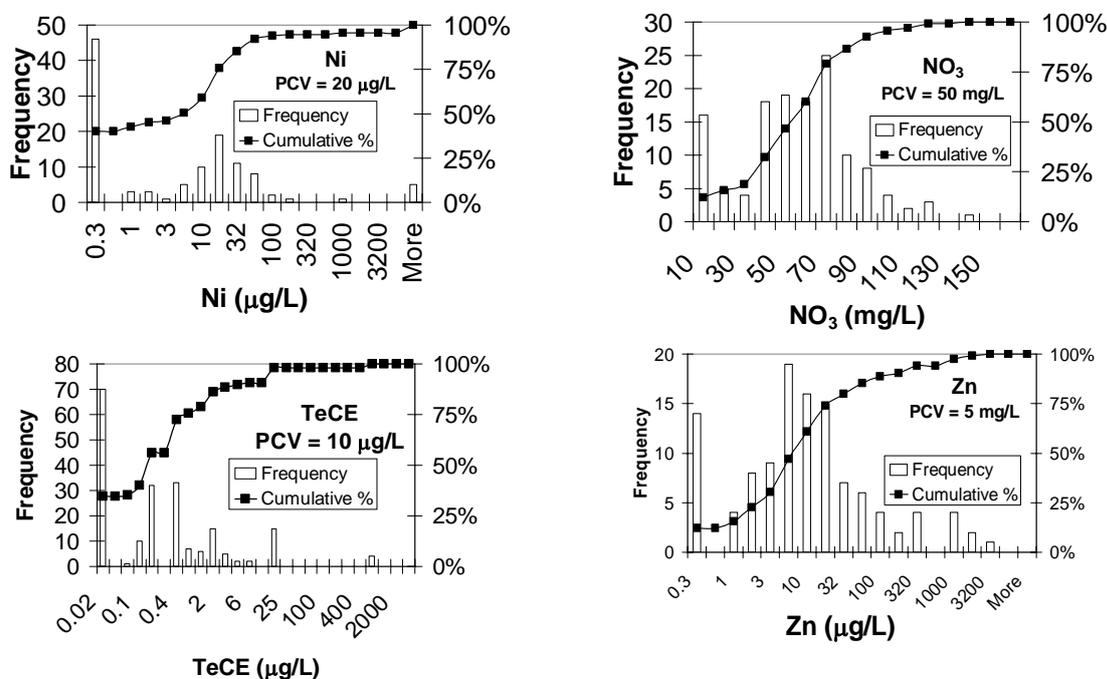
**Fig. 3:** Concentration frequency plots for the (industrial) wellwaters of the unconfined zone for the surveys of Ford & Tellam (1994) and Rivett et al. (1990). All samples included (number ~ 140; 61 wells). PCV = (UK) prescribed conc. or value. From Tellam (In Press).
