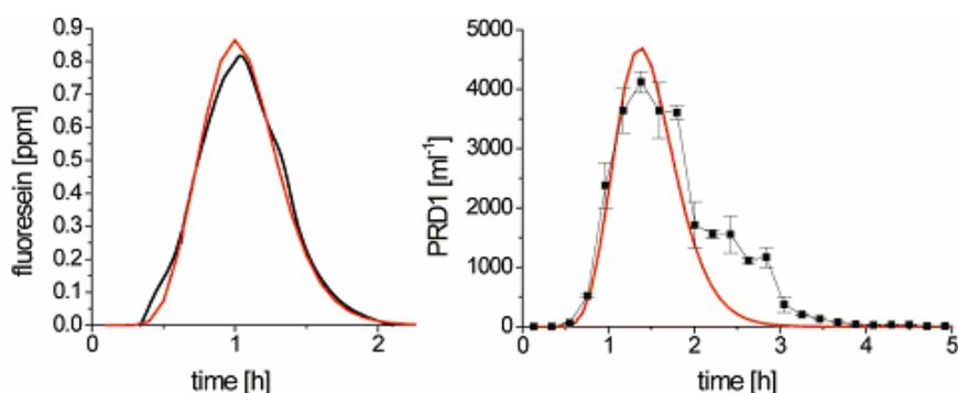
**Fig. 4:** Laboratory experiment on intact sandstone column showing fluorescein and PRD1 breakthroughs (Joyce et al., In Press). Injection concentrations: fluorescein = 1 mg/L; PRD1 = 36,000 pfu/mL. The core is 4.9 cm long. Solid line is a model fit.
