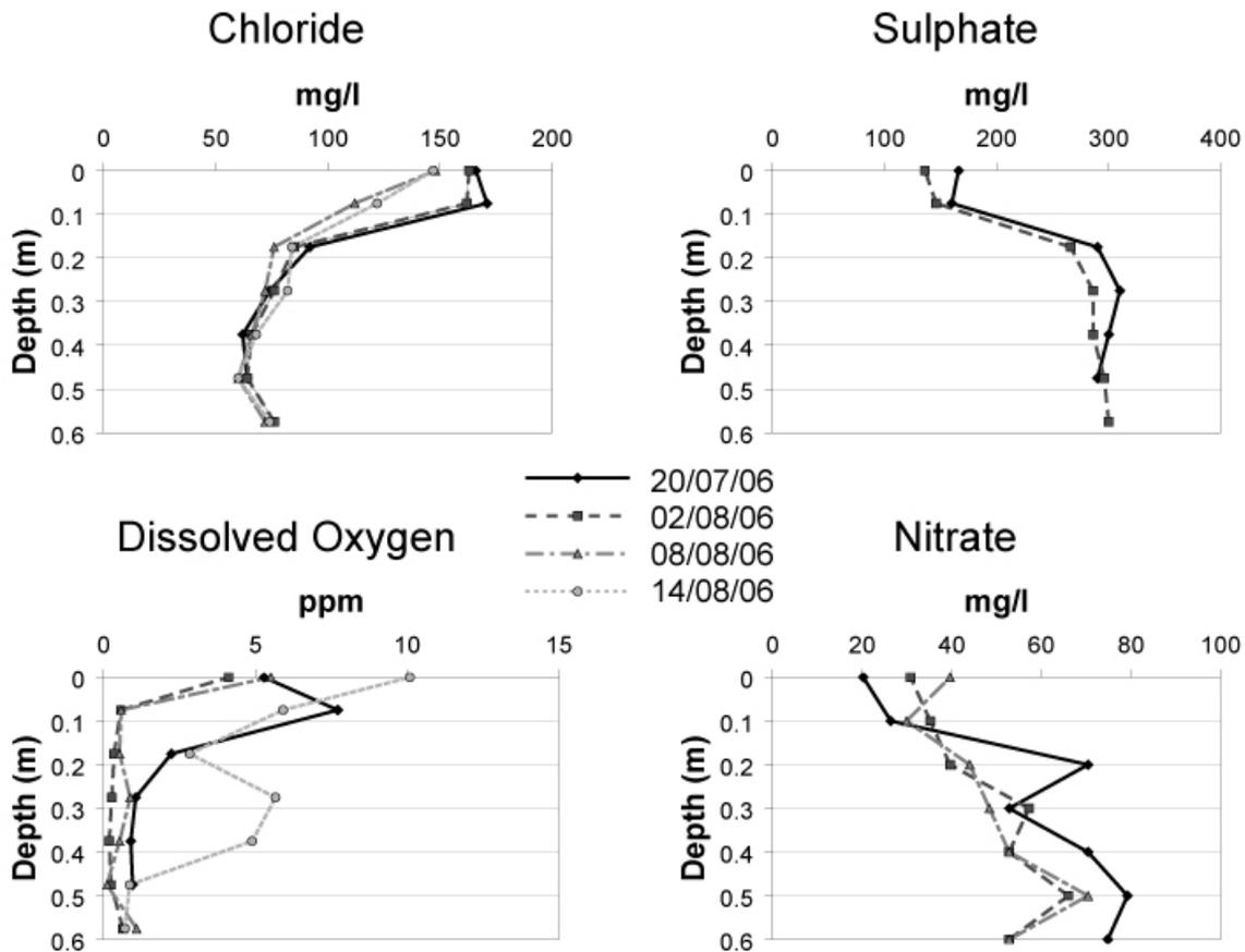
**Figure 2. Chemical riverbed profiles obtained in the River Tame close to the field experiment reach**
