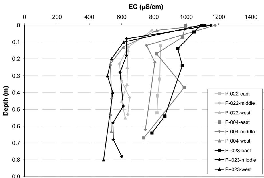
Figure 3. E-W trend recently observed in the conductivity profiles in the transects located 22 m and 4 m upstream and 23 m downstream from the extraction well located on the east bank
