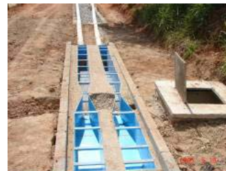
Figure 1: a) Partial view of the contributing area; b) Inflow measurement devices
