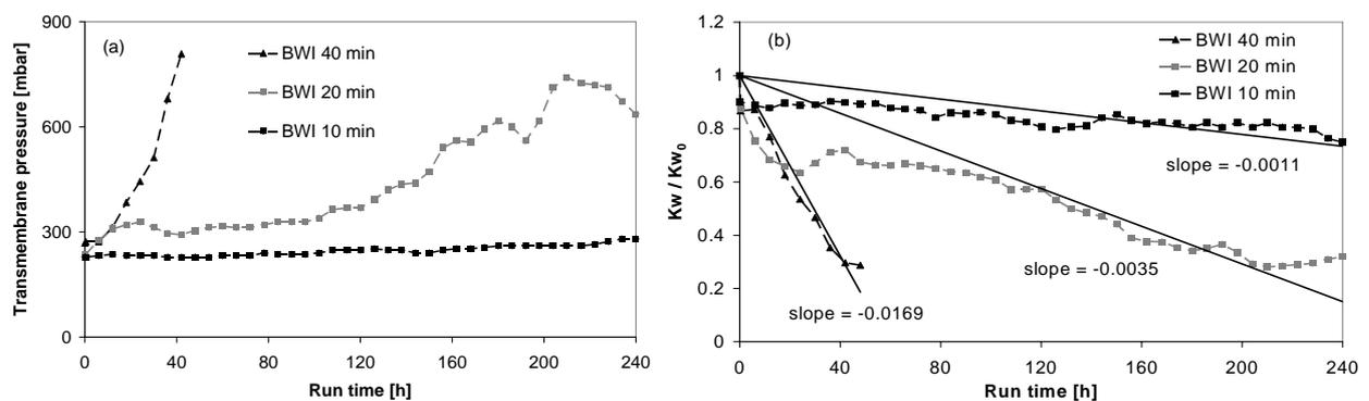
Figure 3: (a) TMP development vs. run time at different BWI (b) Kw/Kw<sub>0</sub> vs. run time at different BWI. Other operating parameters were identical: flux 50 lmh, BWT 20 seconds
