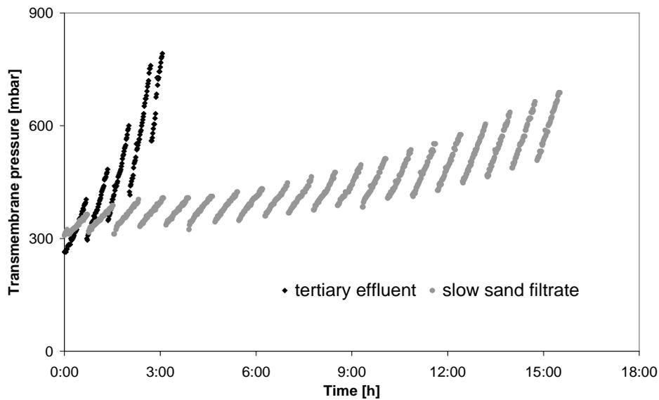
Figure 1: TMP development filtrating tertiary effluent and slow sand filtrate
