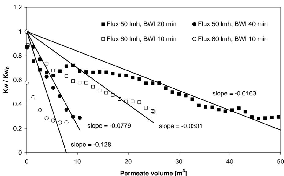
Figure 4: Significance of flux and BWI on membrane productivity reduction
