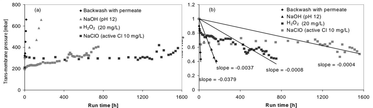
Figure 5: (a) TMP development vs. run time using permeate backwash and enhanced backwash reagents
