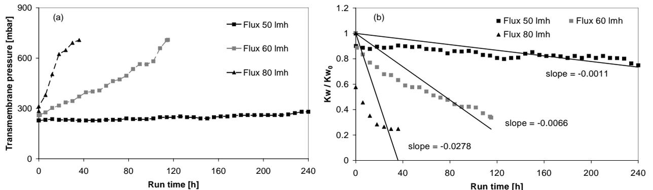
Figure 2: (a) TMP development vs. run time at different fluxes (b)  $K_w/K_{w_0}$  vs. run time at different fluxes. Other operating parameters were identical: BWI 10 minutes and BWT 20 seconds
