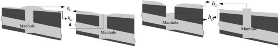
**Figure 2:** (a) Free weir linkage and (b) Submerged weir or orifice linkage.
