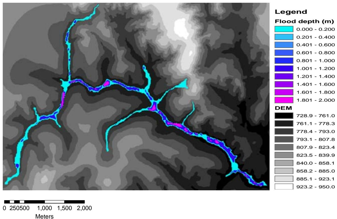
**Figure 7:** Maximum Flood depth for the 1 hour storm
