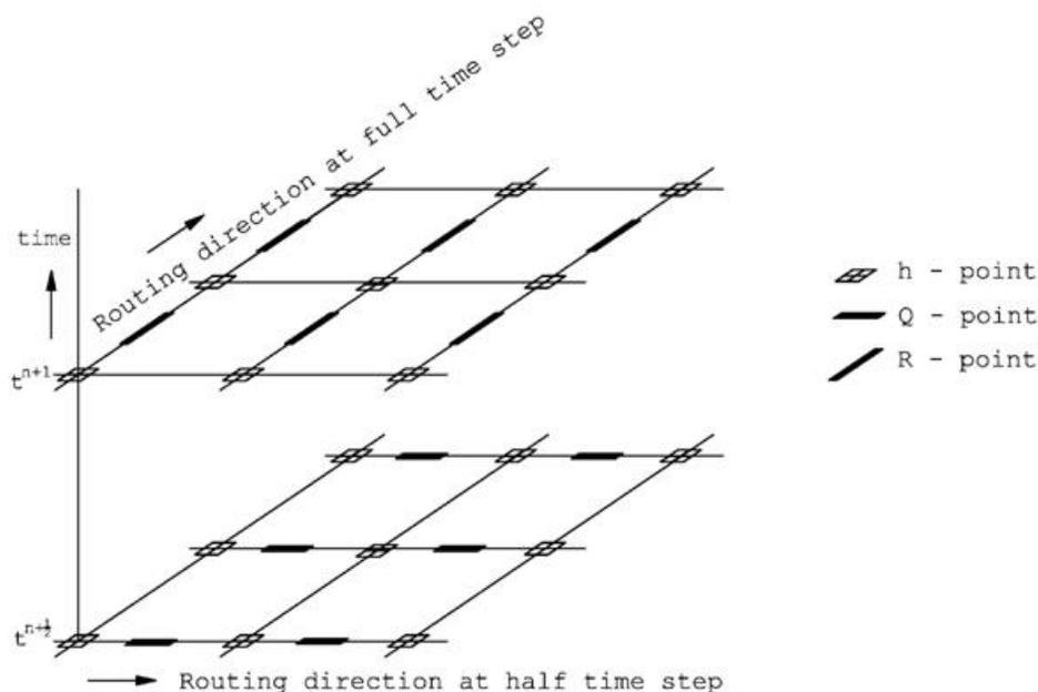
**Figure 1:** Schematic representation of alternating direction flood routing during each half time step.
