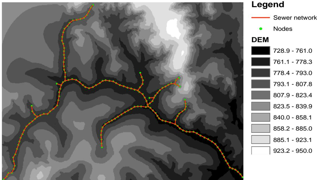
**Figure 6:** Network schematization in Mouse
