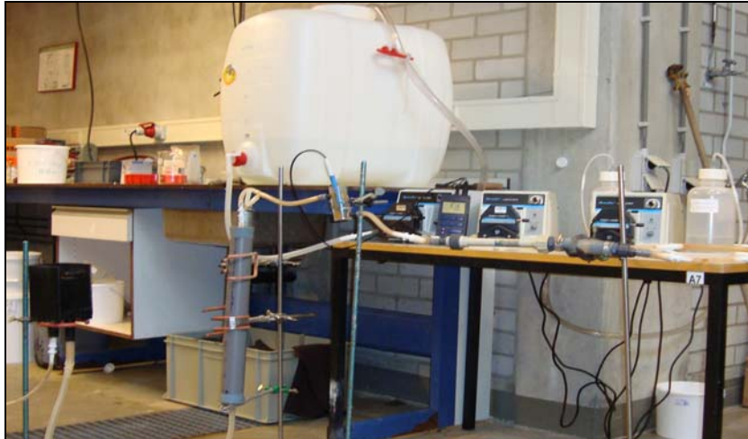
Figure 3-4: Picture of chemical reduction of Cr(VI) to Cr(III) and filter column.
