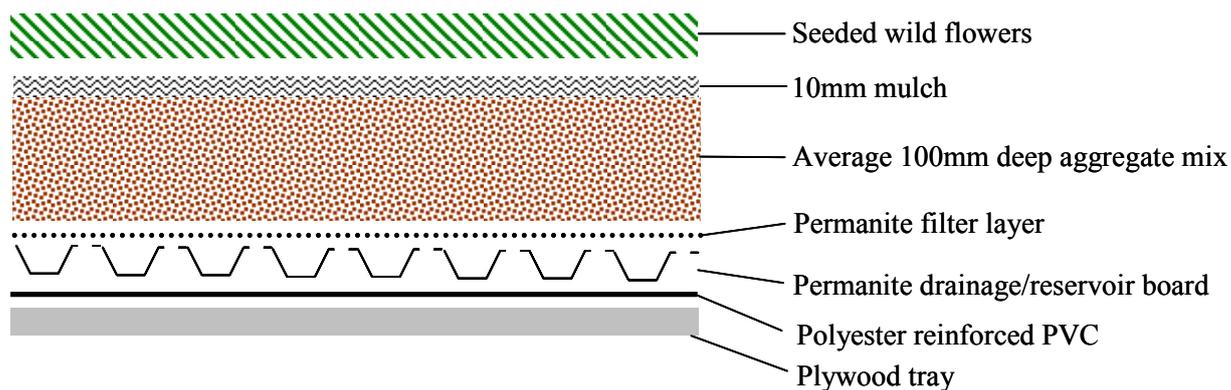
**Figure 3.1.1.1 Schematic diagram of green roof system (Bates et al., 2006)**
