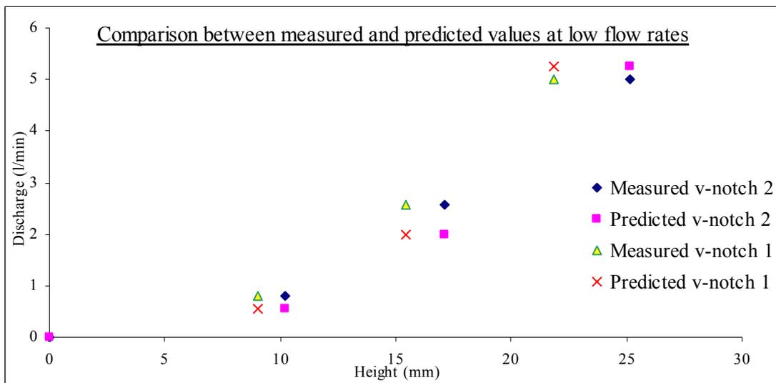
Figure 3.2.3 V-notch weir ultrasonic sensor calibration, comparison of predicted and recorded values
