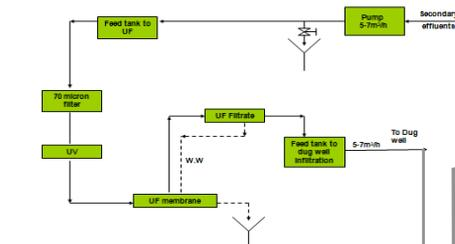
Fig. 2 – RECLAIM pilot plant: UF filtration of secondary effluents
