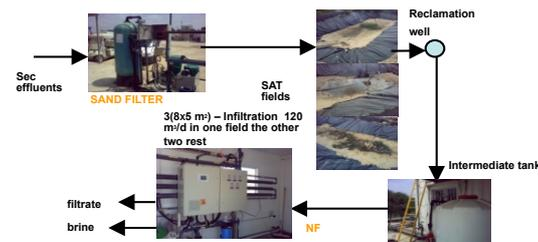
Fig. 4 - SWITCH pilot plant: Sand filter-Short SAT –NF to improve infiltration velocity, organics and micropollutants removal
