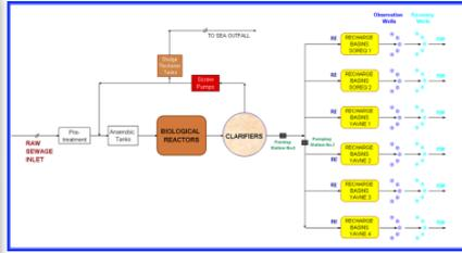
Fig. 1 – Dan Region WWTP and the Soil Aquifer Treatment (SAT)
