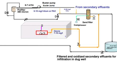
Fig. 3 – OZONATION pilot plant: Improvement of the short SAT anoxic conditions and reduction of manganese dissolution by aeration-sand filtration - ozonation of the secondary effluents (German –Israeli cooperation project)
