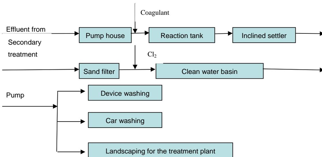
Figure 15. The reclamation procedure for the reclamation at the plant itself
