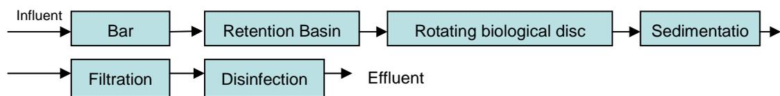
Figure 8. The typical procedure of the typical procedure of rotating biological disc
