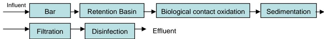
Figure 7. The typical procedure of biological contact oxidation
