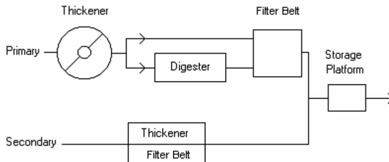
Figure 13. **The sludge treatment at Gaobeidian Sewage Treatment Plant**
