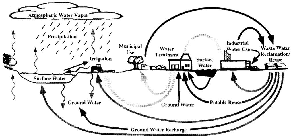
Figure 1 The Role of Engineered Treatment, Reclamation, and Reuse Facilities in the Cycling of Water Through the Hydrologic Cycle (Asano and Levine, 1996)
