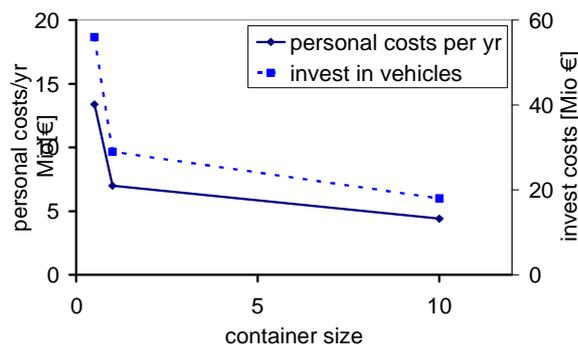
**Figure 10:** Personal and invest costs of truck-based blackwater transport depending on container-size
