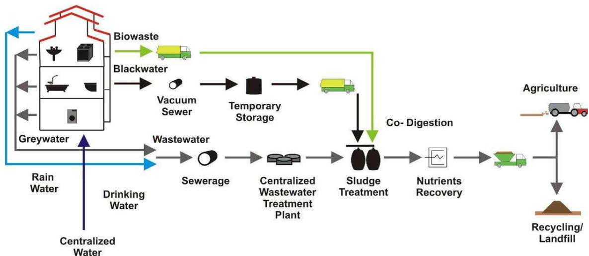
**Figure 1:** Concept of blackwater collection for biogas production, greywater and rainwater collection in sewer system (Meinzinger 2008)
