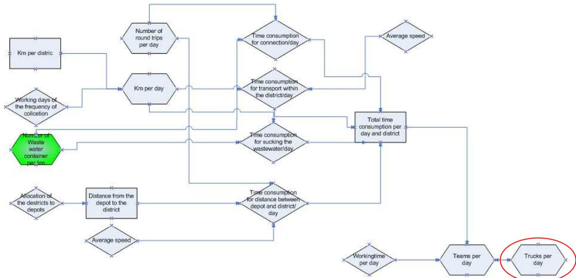
**Figure 6:** Flow diagram for finding number of trucks required
