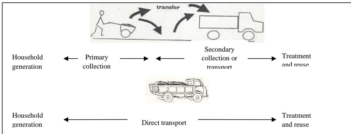
**Figure 2: Example of transport with transfer and direct transport**
