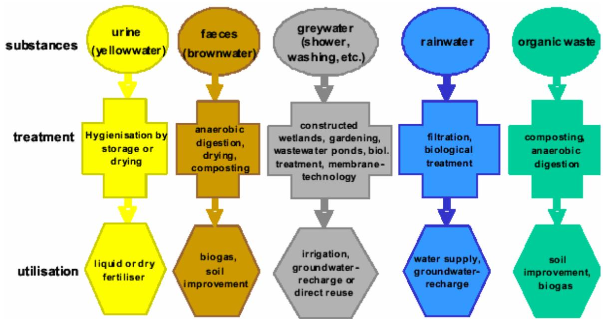
**Figure 7. Separation of substances and options for treatment and utilization**
