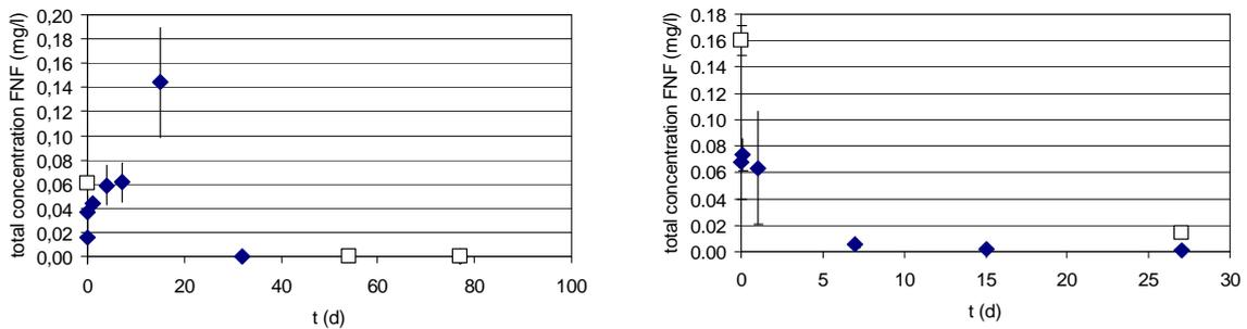
**Figure 5.21:** Fenofibrate (FNF) concentration in time of the anaerobic experiments ANAER-1 (left) and ANAER-2 (right) (♦ with sludge, □ without sludge).
