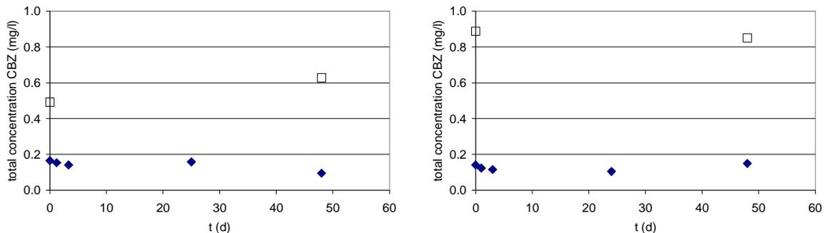
**Figure 5.18.** Total concentration of carbamazepine (CBZ) in time in the anoxic test at 10 °C (ANOX-10, left) and 20°C (ANOX-20, right) batch tests (♦ with sludge, □ without sludge)
