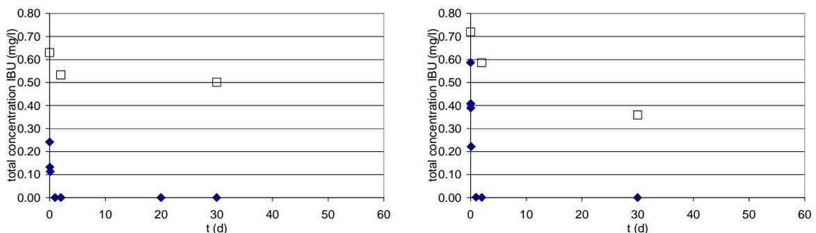
**Figure 5.6:** Total concentration of ibuprofen (IBU) in the aerobic test at 20°C (AER-20-2, left) and 10°C (AER-10, right). (◆ with sludge, □ without sludge)
