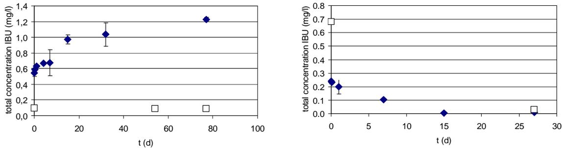
**Figure 5.22:** Ibuprofen (IBU) concentration in time of the anaerobic experiments ANAER-1 (left) and ANAER-2 (right) (♦ with sludge, □ without sludge).
