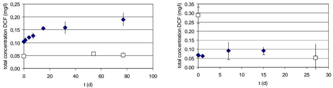
**Figure 5.25:** Diclofenac (DCF) concentration in time of the anaerobic experiments ANAER-1 (left) and ANAER-2 (right) (◆ with sludge, □ without sludge).
