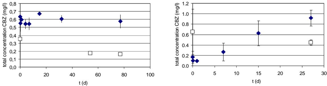
**Figure 5.26.** Carbamazepine (CBZ) concentration in time of the anaerobic experiments ANAER-1 (left) and ANAER-2 (right) (◆ with sludge, □ without sludge).
