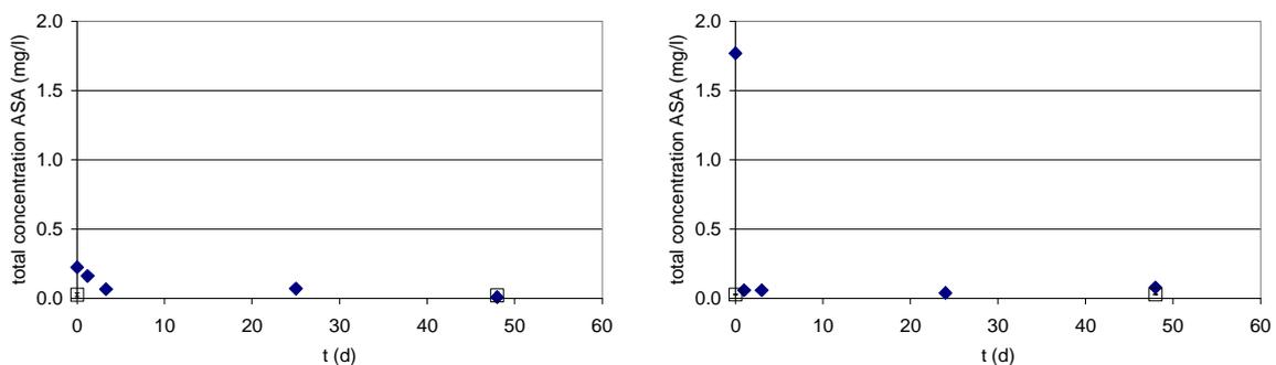
**Figure 5.12:** Total concentration of aspirin (ASA) in time in the anoxic test at 20 °C (ANOX-20, left) and 10°C (ANOX-10, right) batch tests (◆ with sludge, □ without sludge).
