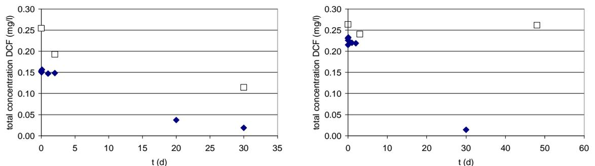
**Figure 5.9:** Concentration diclofenac (DCF) in time in the aerobic test at 20 °C (AER-20-2, left) and at 10°C (AER-10, right). (◆ with sludge, □ without sludge)
