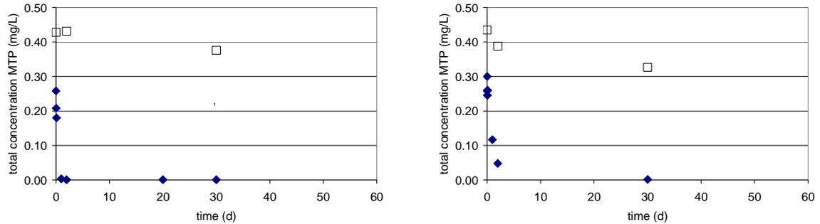
**Figure 5.7:** Concentration of metoprolol (MTP) in the aerobic test at 20°C (AER-20-2, left) and 10°C (AER-10, right). (◆ with sludge, □ without sludge)
