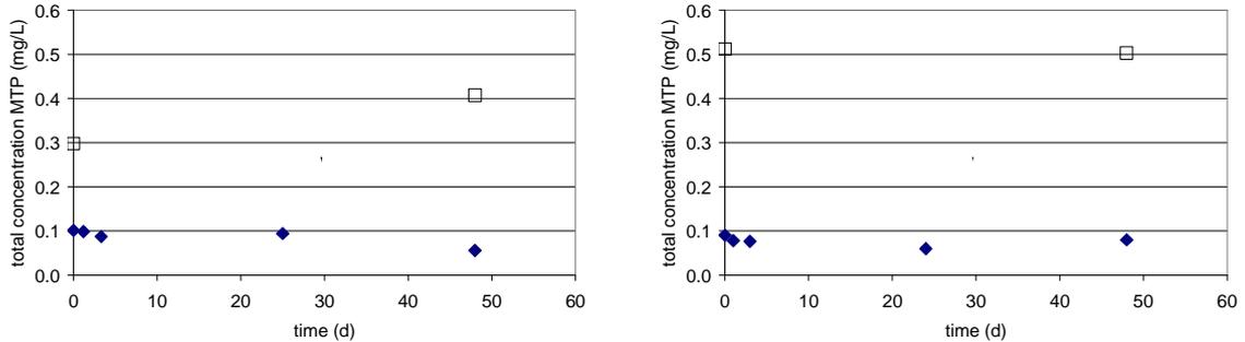
**Figure 5.15.** Total concentration of metoprolol (MTP) in time in the anoxic test at 10 °C (ANOX-10, left) and 20°C (ANOX-20, right) batch tests (♦ with sludge, □ without sludge)
