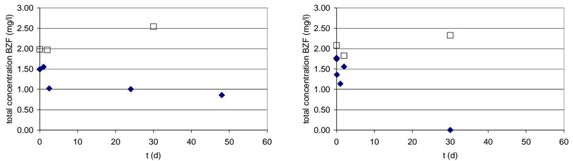
**Figure 5.8:** Concentration bezafibrate (BZF) in time in the aerobic test at 20 °C (AER-20-2, left) and at 10°C (AER-10, right). (◆ with sludge, □ without sludge)
