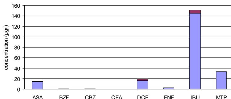
**Figure 5.2.** Background concentration of pharmaceuticals in anaerobic sludge sampled from pilot-scale UASB reactor fed with concentrated black water investigated in Leeuwarden, the Netherlands (de Graaff et al., 2008). Liquid and solid fraction are distinguished; the darker color indicates pharmaceutical compounds in solid fraction.
