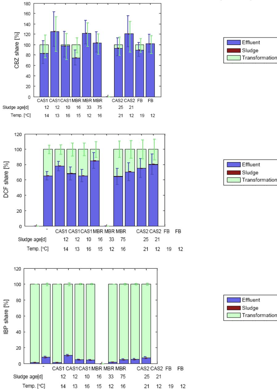
**Figure 3.5.** Removal of pharmaceutical compounds in full scale conventional activated sludge, membrane bioreactor and fixed bed reactor systems (Joss 2005); CBZ; carbamazepine, DCF; diclofenac, IBP; ibuprofen.
