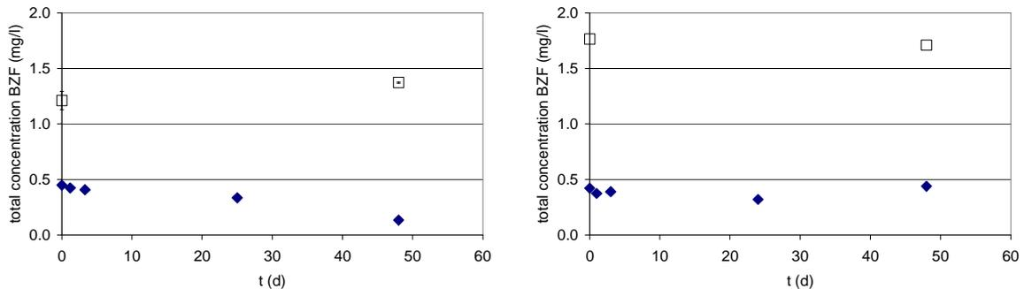
**Figure 5.16.** Total concentration of bezafibrate (BZF) in time in the anoxic batch test at 10 °C (ANOX-10, left) and 20°C (ANOX-20, right) batch tests (♦ with sludge, □ without sludge)
