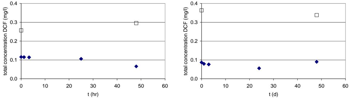
**Figure 5.17:** Total concentration of diclofenac (DCF) in time in the anoxic test at 10 °C (ANOX-10, left) and 20°C (ANOX-20, right) batch tests (♦ with sludge, □ without sludge)
