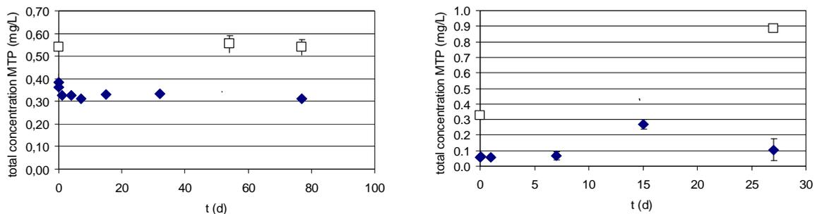
**Figure 5.23:** Metoprolol (MTP) concentration in time of the anaerobic experiments ANAER-1 (left) and ANAER-2 (right) (◆ with sludge, □ without sludge).
