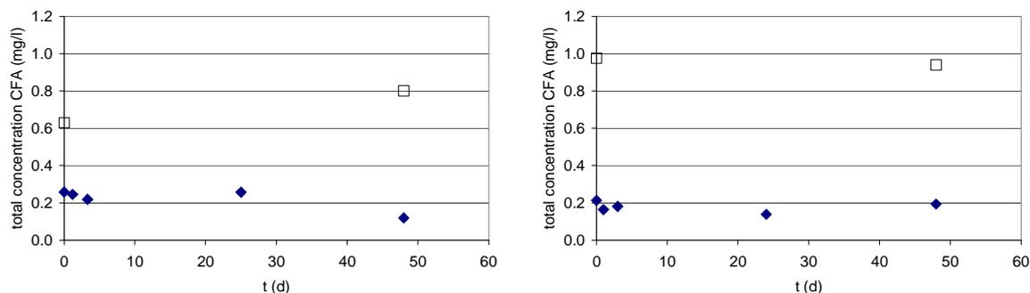
**Figure 5.19.** Total concentration of clofibric acid (CFA) in time in the anoxic test at 10 °C (ANOX-10, left) and 20°C (ANOX-20, right) batch tests (♦ with sludge, □ without sludge)
