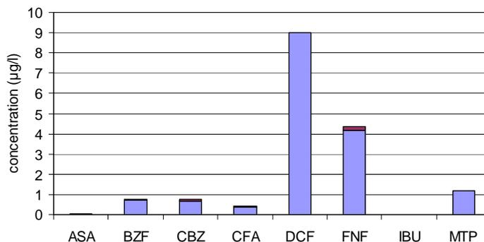
**Figure 5.1:** Background concentration of selected pharmaceuticals in activated sludge mixture of municipal WWTP Bennekom. Liquid and solid fraction are distinguished; the darker color indicates pharmaceutical compounds in solid fraction. Presented data is obtained from three activated sludge samples taken in January and February 2008.
