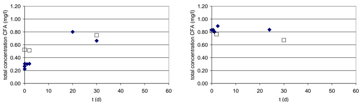
**Figure 5.11.** Concentration clofibric acid (CFA) in time in the Aerobic test at 20°C (AER-20-2, left) and at 10°C (AER-10, right). (◆ with sludge, □ without sludge)
