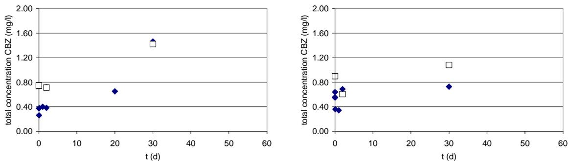
**Figure 5.10.** Concentration carbamazepine (CBZ) in time in the aerobic test at 20 °C (AER-20-2, left) and at 10°C (AER-10, right). (◆ with sludge, □ without sludge)
