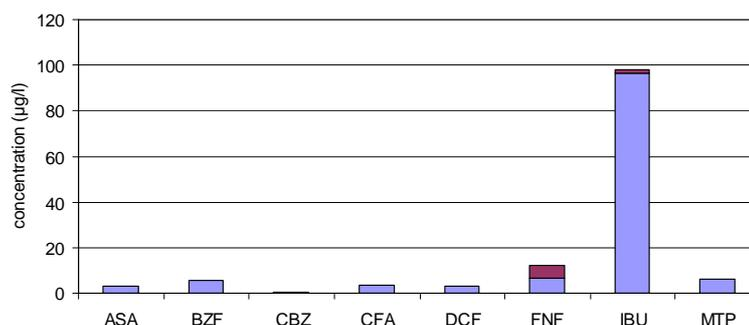
**Figure 5.3:** Background concentration of pharmaceuticals in anaerobic sludge obtained from demonstration-scale UASB septic tank treating concentrated black water (the same as the pilot-scale UASB, Leeuwarden) in Sneek, the Netherlands. Liquid and solid fraction are distinguished; the darker color indicates pharmaceutical compounds in solid fraction.
