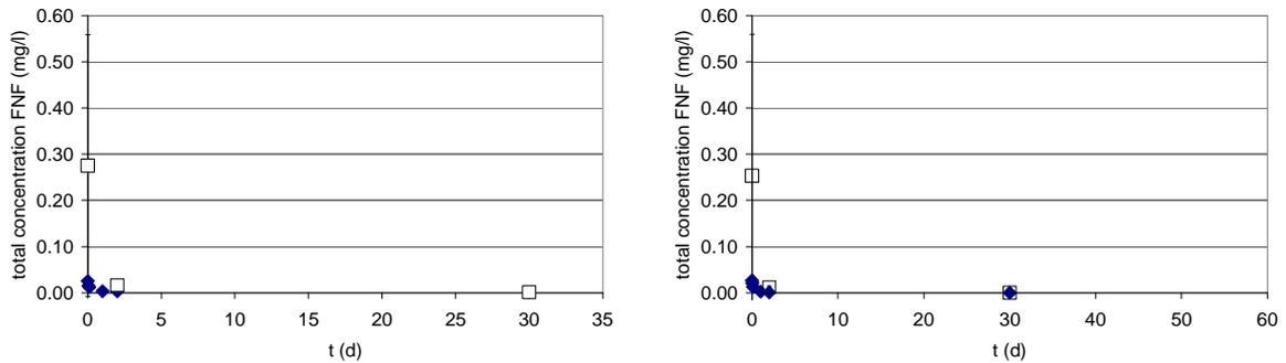
**Figure 5.5:** Total concentration of fenofibrate (FNF) in time in the aerobic batch test at 20°C (AER-20-1, left) and at 10°C (AER-10, right). (◆ with sludge, □ without sludge)
