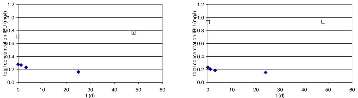
**Figure 5.14.** Total concentration of ibuprofen (IBU) in time in the anoxic test at 10 °C (ANOX-10, left) and 20°C (ANOX-20, right) batch tests (♦ with sludge, □ without sludge)
