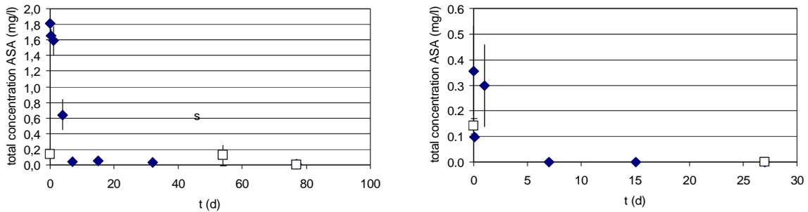
**Figure 5.20:** Aspirin (ASA) concentration in time of the anaerobic experiments ANAER-1 (left) and ANAER-2 (right) (♦ with sludge, □ without sludge).
