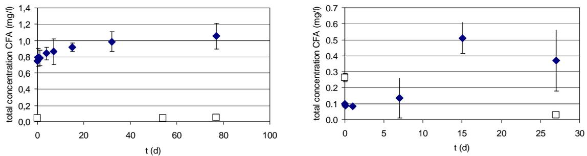
**Figure 5.27:** Clofbric acid (CFA) concentration in time of the anaerobic experiments ANAER-1 (left) and ANAER-2 (right) (◆ with sludge, □ without sludge).
