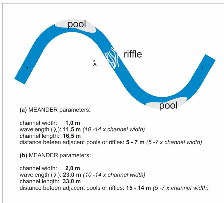
Figure 5. Models of meanders applied in the Sokołówka rehabilitation project: (a) parameters for model of meander for 1m width river, (b) parameters for model of meander for 2m width river (after Leopold and Langbein 1966, changed) Pool-riffle sequence formation
