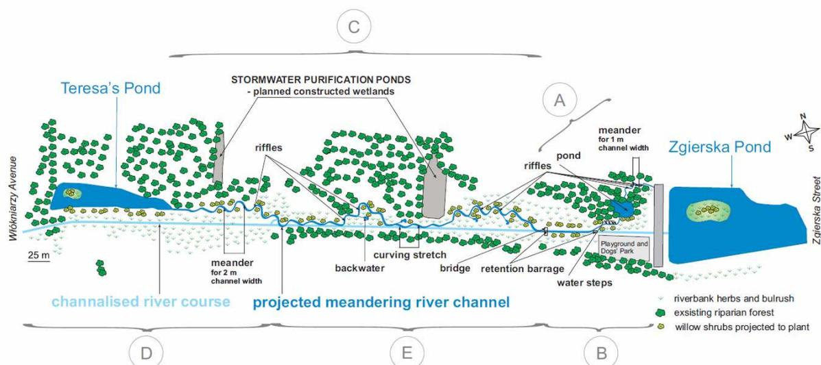
Figure 4. The Sokołówka rehabilitation project design (modified from Zalewski et al. 2009 and Łapińska et al. 2010)
