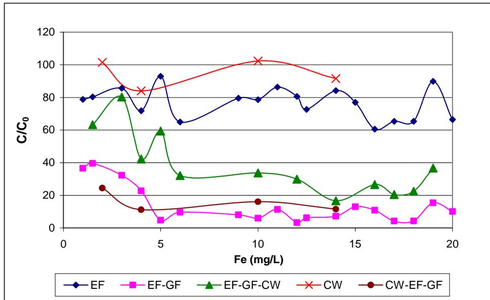
Figure 4: Residual phosphorus in ‘Shafdan’ secondary effluent for different treatments.  $C_0=1-3$  mg/l TP. Flow rate  $1.5$  m<sup>3</sup>/hr.
