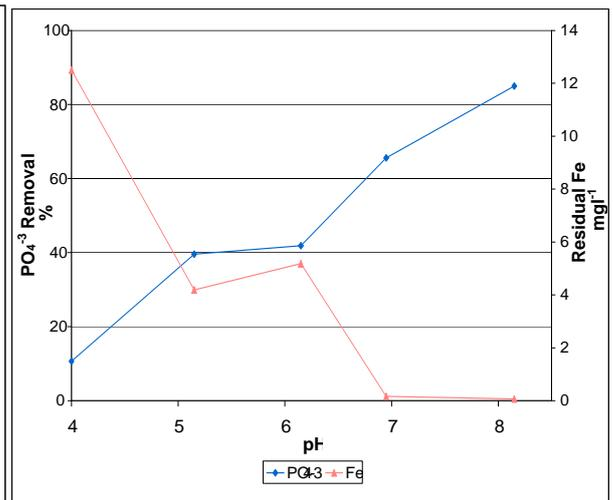
Figure 2: Phosphate removal by a modified jar-test as a function of pH of pH
